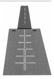
This pattern helps the pilot to judge the aircraft's height and to line up with the runway on the approach to land. In addition, these high- intensity white lights are invaluable in conditions of poor visibility by day, as well as at night, in helping the pilot to find the approach path visually, towards the end of a radio or radar-controlled approach.
