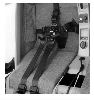
14. <u>Fitting</u>. To fit the aircraft safety harness, loosen off the adjustable straps and insert the four adjustable harness lugs.
