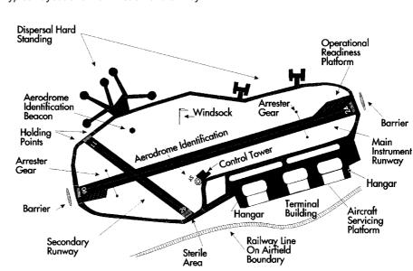
Fig 1-1 Typical layout of a main instrument runway
