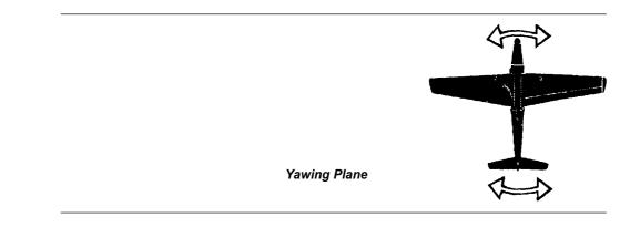
(2) <u>Rudder Pedals</u>. The rudder is operated by the pilot's feet and causes the aircraft "yaw" – that is to turn without banking. The rudder is used a lot during aerobatics, but for most normal flying its main purpose is to maintain balanced flight.
