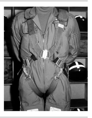
9. <u>Adjustment</u>. There are four adjusters on the harness to allow for different body sizes but the majority of adjustment is done by lengthening or shortening the leg straps.
