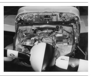
5. <u>GROB 2500 E1 Engine</u>. Power is provided by a GROB 2500 E1 horizontallyopposed 4-cylinder air-cooled petrol engine, developing 95 BHP at 3400 rpm.
