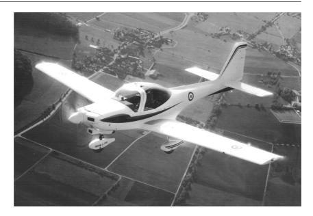
Length 7.6m Height 2.4m Max all-up mass 990kg Engine Lycoming 180hp Never exceed speed (VNE) 185kts
